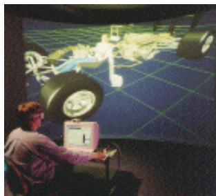
A SEMI-IMMERSIVE WIDE-SCREEN PROJECTION SYSTEM IN USE WITH SHUTTER GLASSES
