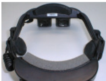
The major components of an HMD. This illustration shows the two screens capable of producing stereo images and speakers located to provide stereo sound.
